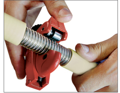
2. Cut the hose to the required size in the middle of two corrugations.
