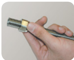
2. Slide the nut over the hose
