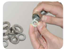
5. Insert the gasket
