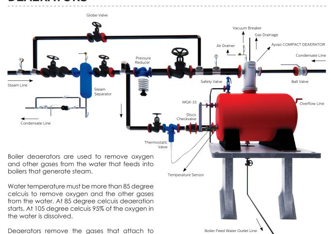
the metallic components of the steam system and cause corrosion by forming oxides, or rust. Oxygen and carbon dioxide are responsible for corrosion(pitting). There are two types of boiler deaerators: Tank model or compact deaerators.
