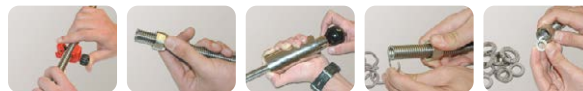
1. Measuring and cutting the hose 2. Slide the nut over the hose 3. Press the piston 4. Fit the clamping washer 5. Insert the gasket
